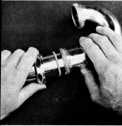
A flexible-ring compression joint. When the parts of this joint are in good condition, the flange nut need be no more than finger-tight to hold water.
