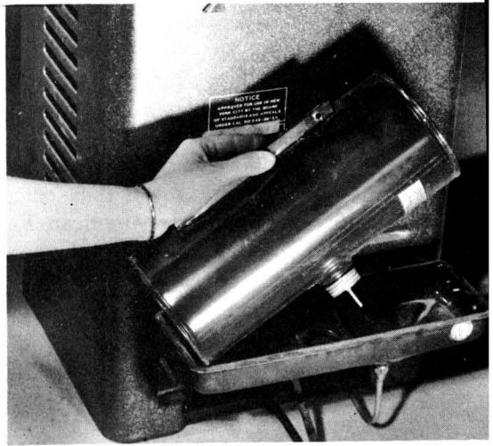
"Atmospheric" type of fuel-supply tank for small portable or vented oil space heater. Pin protruding from tank cap is part of valve that is spring-closed when tank is lifted out of oil reservoir below it. When tank is set down in reservoir pin is pushed upward by contact with bottom of reservoir, releasing oil into reservoir.
